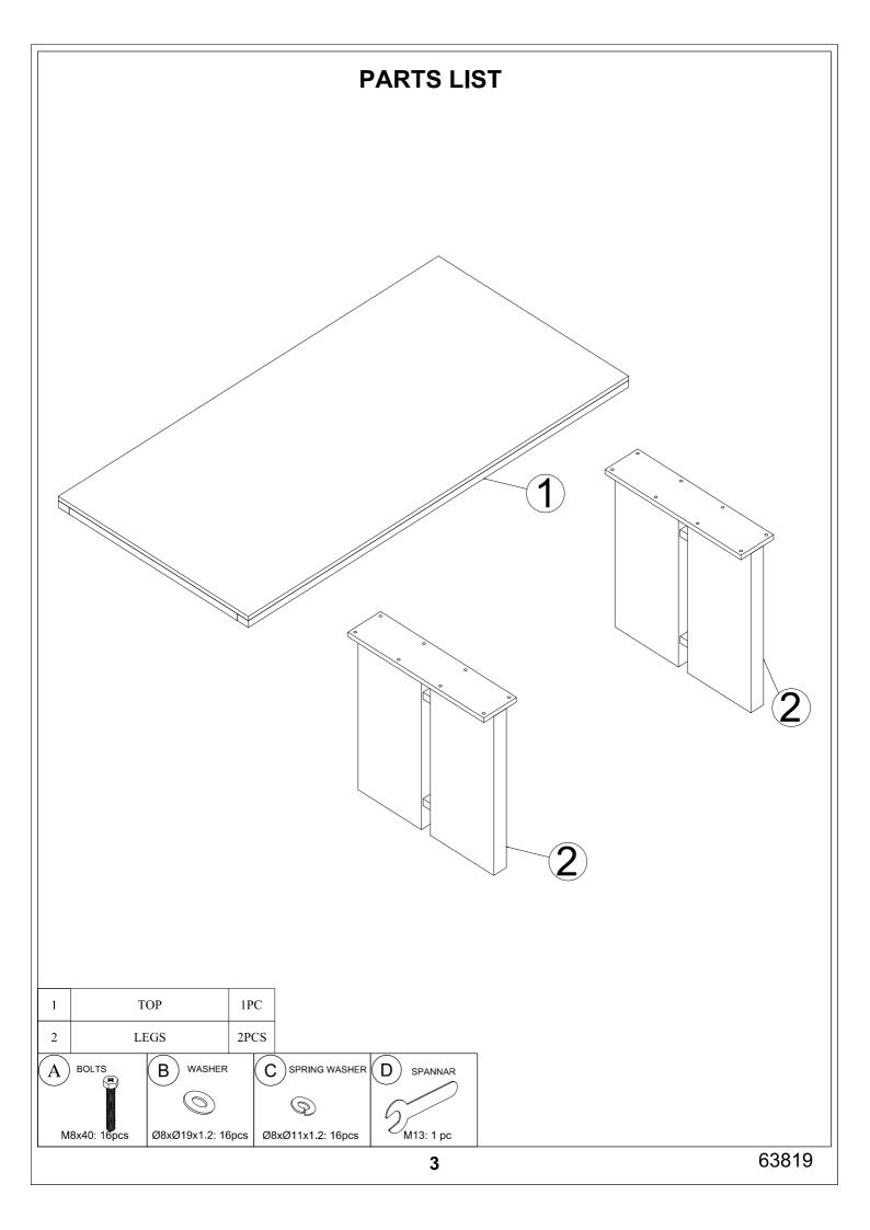
Step 1: Fasten the legs (2) To the top (1) with bolts (A), washer (B), spring washer (C) and using spannar (D)
